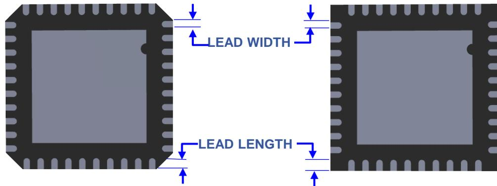
**Exposed Pad, Lead Length and Lead Width dimensions remains within tolerance.**
